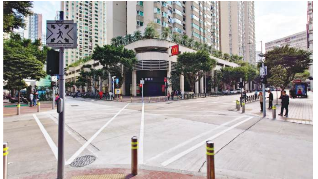
This handout photo provided by the Transport Bureau (DSAT) yesterday shows the diagonal crossing at the junction of Rua Nova da Areia Preta (黑沙環新街) and Rua de Ma Kau Seak (馬交石街).
