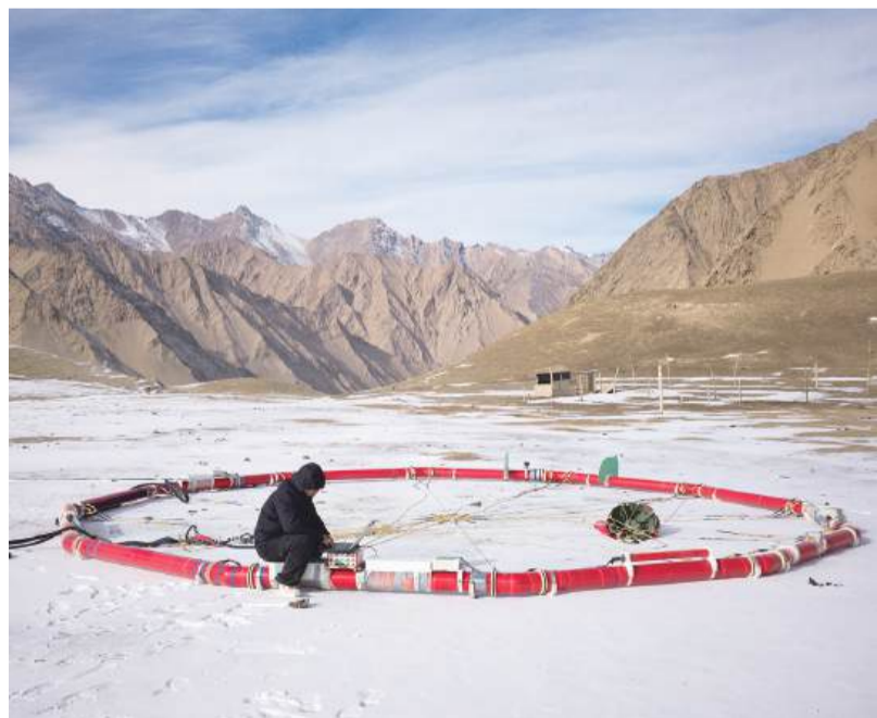
A researcher tests a helicopter airborne magnetotelluric detection (HAMT) system in Hetian, Xinjiang Uygur Autonomous Region, last month. China's first helicopter airborne magnetotelluric detection system has been successfully applied to a plateau railway construction project, the Chinese Academy of Sciences' Aerospace Information Research Institute (AIR) said yesterday. The HAMT system is a geophysical survey technology used in mineral exploration, geological mapping, and environmental studies. "Telluric" refers to phenomena related to the Earth. — Xinhua/Poe
